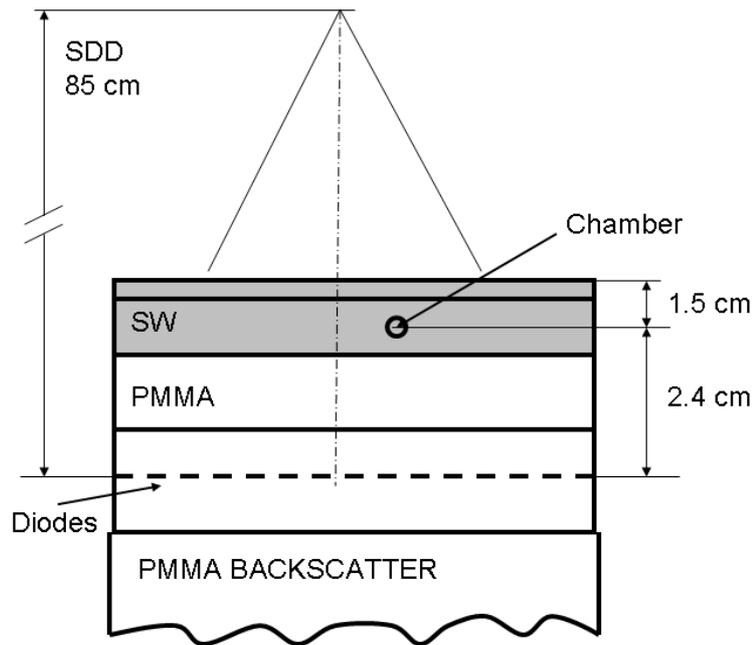
**Figure 2.** Experimental setup for measurements with the detector board in the calibration phantom with an ion chamber reference.
