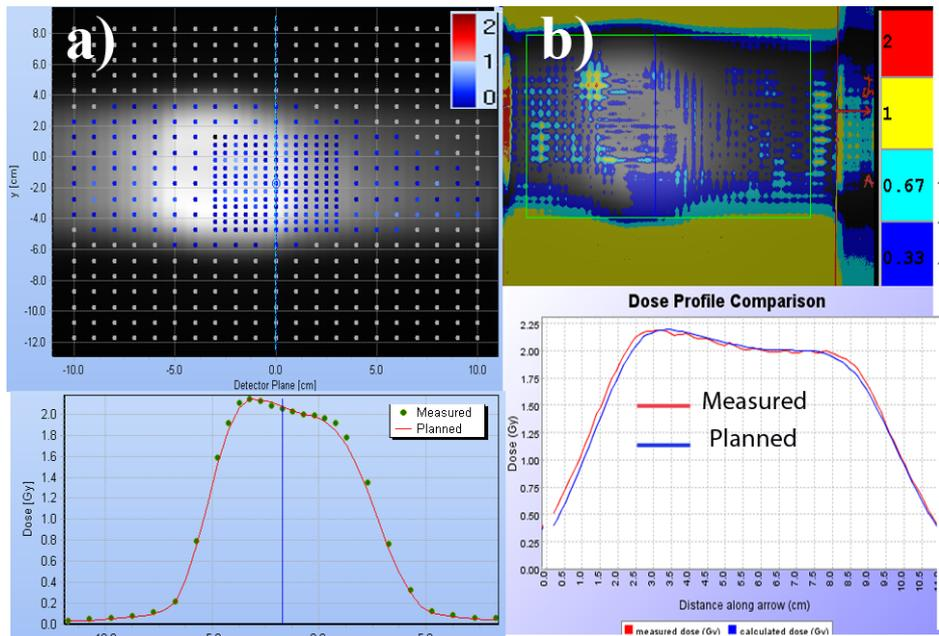
**Figure 4.** Dose comparison for Case 7 in the sagittal plane (main board). a) Delta4 vs. planned (absolute). b) Film vs. planned (relative). Top:  $\gamma(3\%,3\text{mm})$ . Bottom: longitudinal dose profiles.
