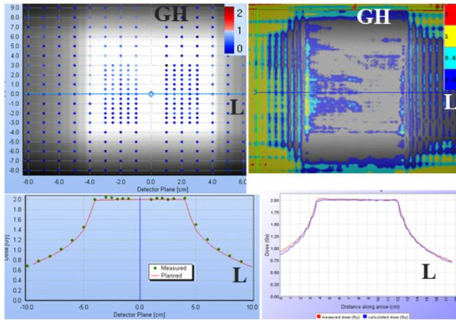
**Figure 3.** Gamma maps (top) and transverse dose profiles (bottom) comparing measured and calculated doses for Delta4 (left) and film (right) in the coronal plane (wings).  $\gamma(3\%/3\text{mm})$  is used for the absolute Delta4 dose comparison and  $\gamma(2\%/2\text{mm})$  for the relative film comparison.
