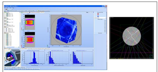
Fig 4: Measurement compared to calculations for the Simple Model. Scan of DELTA4 with the CT table model (bright lines represent the detector planes, density overwritten in TPS).
