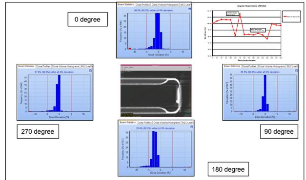
Fig 1: Comparison of calculated (uncorrected for attenuation) and measured dose for a four field box (0°, 90°, 180°, 270° gantry angle) shown as gamma index. The shift of the gamma index for the 180° radiation shows the expected attenuation by the treatment couch. Directional dependency of the radiation dose measurement at the central detector. CT scan of the accelerator table top imported in the Pinnacle treatment planning system.
