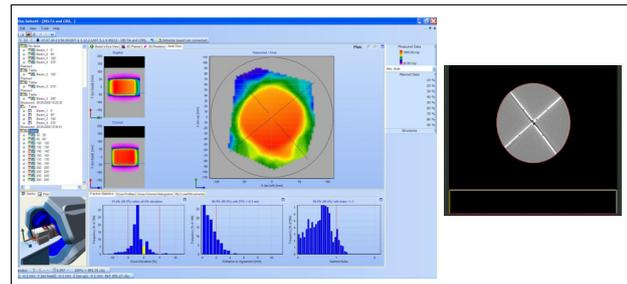
Fig 3: Measurement compared to calculations for the CT Model. Scan of DELTA4 with the CT table model (bright lines represent the detector planes, density overwritten in TPS).
