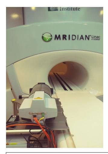
Figure 1. Delta<sup>4</sup> Phantom+ MR. A portable table is included for transportation and easy placement onto the LINAC couch.
