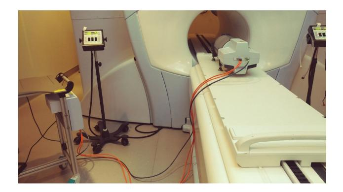
Figure 2. Delta<sup>4</sup> system setup for measurement
