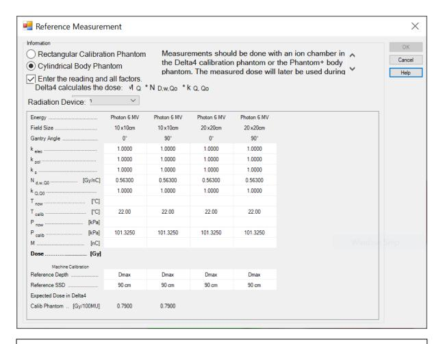
Figure 3. Delta<sup>4</sup> calibration window
