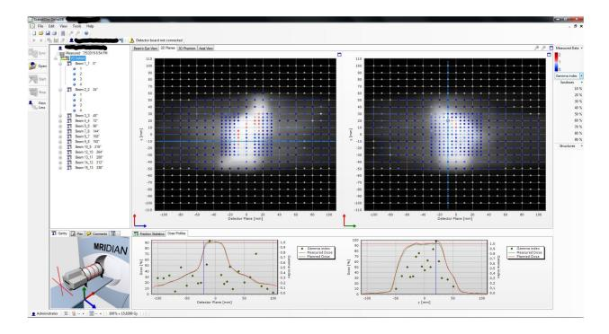
Figure 6. Delta<sup>4</sup> main windows showing for each detector plane ("X"-plane on the left, "Y"-plane on the right). The comparison between the measured dose and the planned dose is showed. The dots represent the value of the Gamma Index according to the right ordinate axis values.
