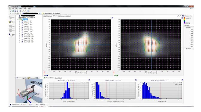
Figure 5. Delta<sup>4</sup> main window showing the pass rates histograms for the absolute dose, Distance-to-Agreement (DTA) and Gamma Index
