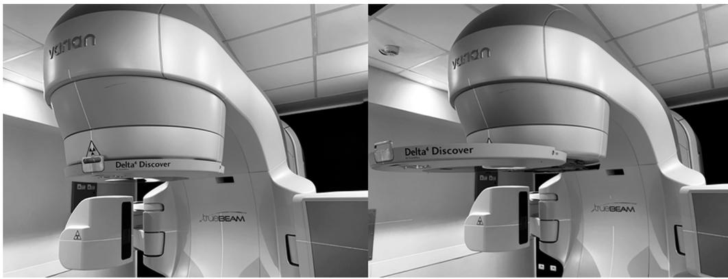
Fig. 1. Delta<sup>4</sup> Discover mounted on the TrueBeam Linac head (left) and slid out while remaining fixed to the gantry (right).
