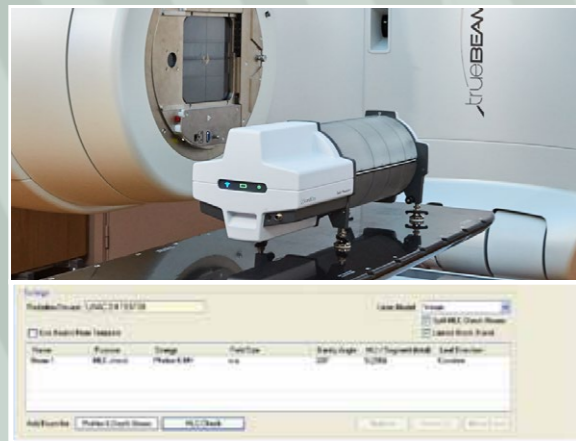
Create a DICOM RT Plan file that includes all QA in one routine, including MLC QA.
