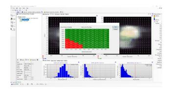
Instant display of dose deviation, distance to agreement, gamma pass rate, and plan pass/fail status
